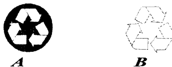
Fig. 6.6 Signs that indicate the possibility of reprocessing of material of the item or presence of reprocessed components in it: A – the product may be reprocessed, B – the product contains the reprocessed materials
