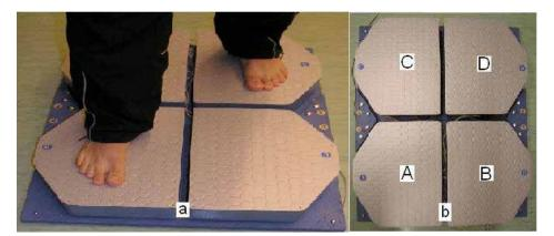
**Figure 1.** Two twin platforms kinesis-meter CQStab2P used for measurements [16]: testing in A–D feet situation (a), plates – sight from above (b).
