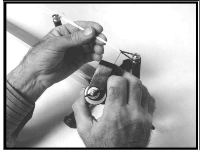
When the correct length of serving has been reached, turn the string jig posts and continue to serve
